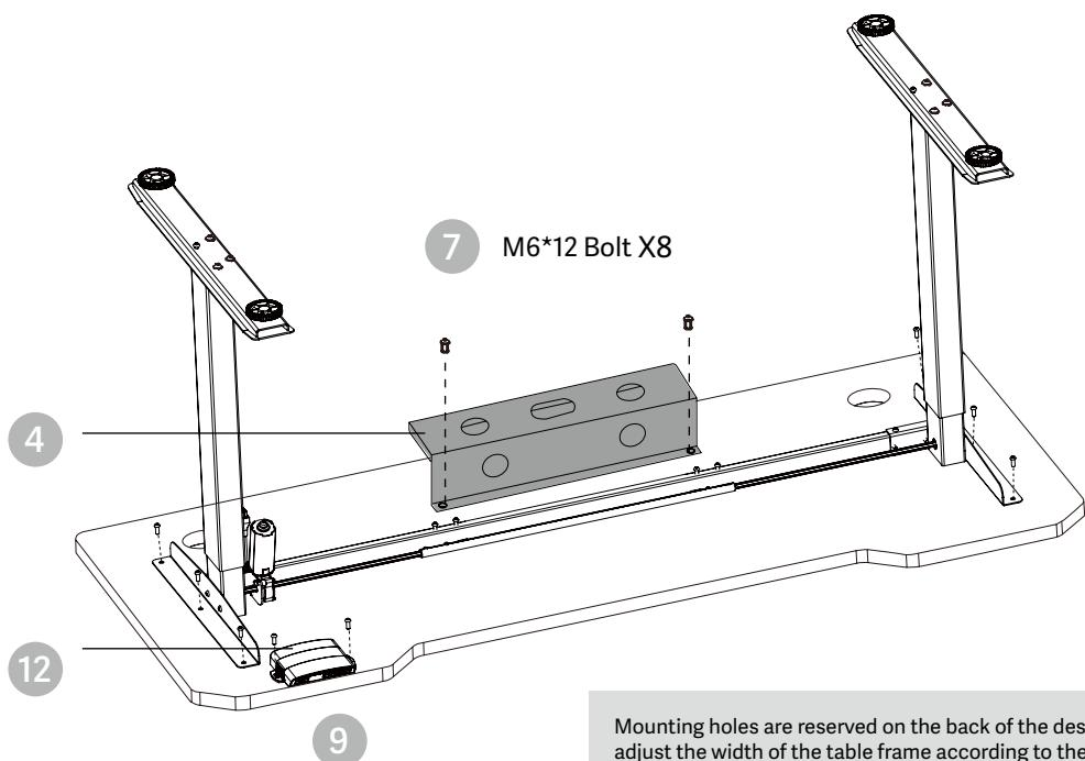
Mounting holes are reserved on the back of the desktop. Please adjust the width of the table frame according to the position of the mounting holes.
