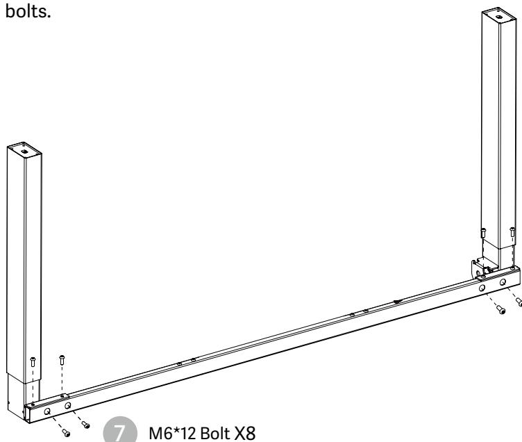
NOTE: Avoid excessive tightening bolts
