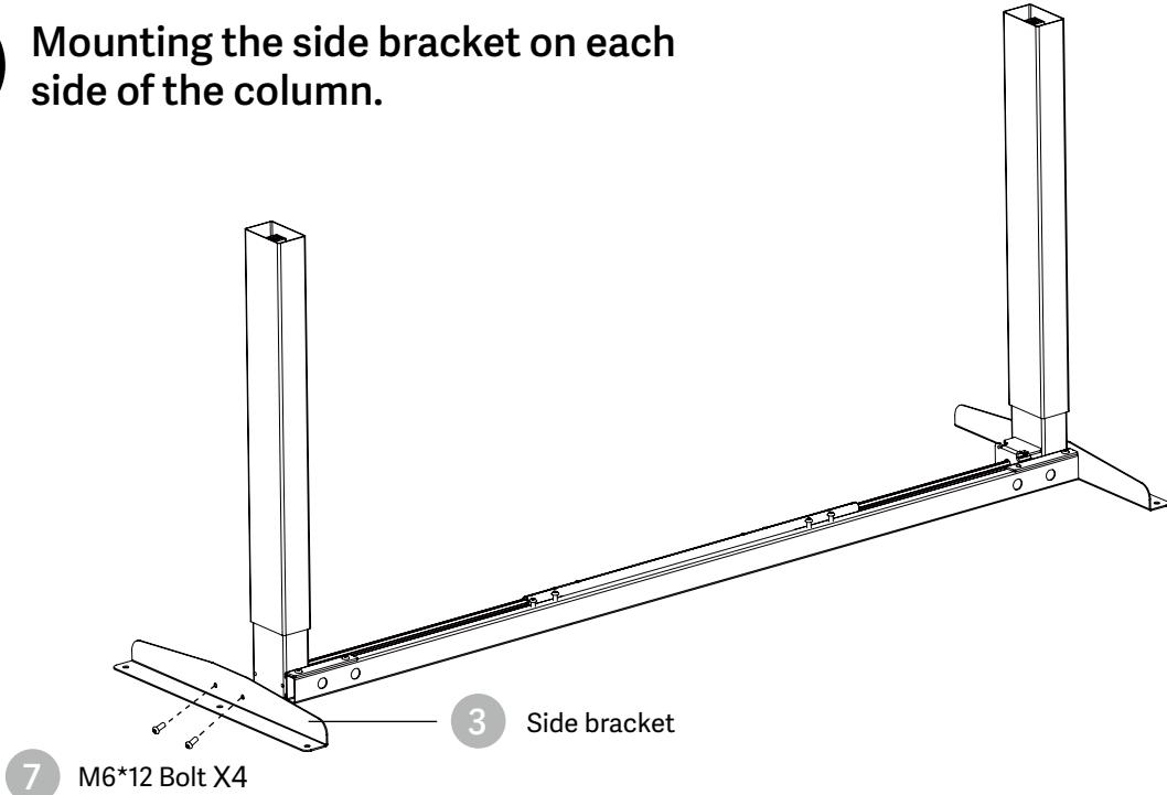
NOTE: Avoid excessive tightening bolts
