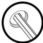
Make sure that the hexagon bar is fully inserted and the groove on the hexagon bar completely sunk into the hexagon hole of the column
